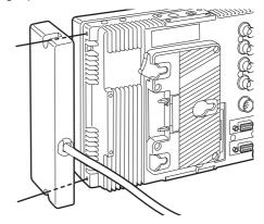
**5** Plug the cord connecting the main controls into the connector on the main unit and secure it.
